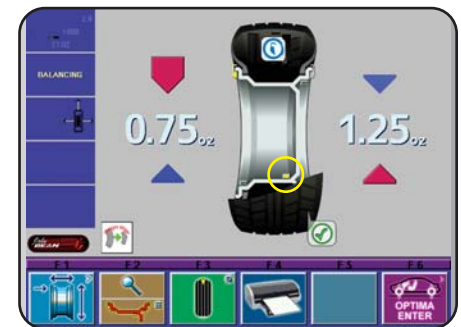
Tape weight and clip weight combination (tape weight location circled in yellow)
